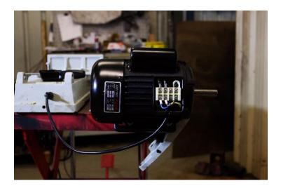
8. Remove 3 wires and twist cable lock 90° to remove.
