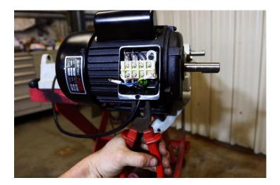
9. Flip base over and loosen all clips and glands holding the wires.
