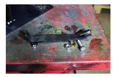
28. Use M12x35mm bolt in the guide adjuster slot, from the inside of the saw.
