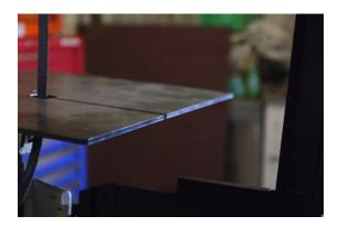
31. Re fit and tension blade, replace blade cover.
