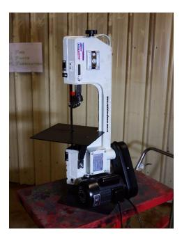
33. Secure mount base to sturdy work bench or platform using 4 (four) suitable bolts (not supplied) in the corners of the base plate.
