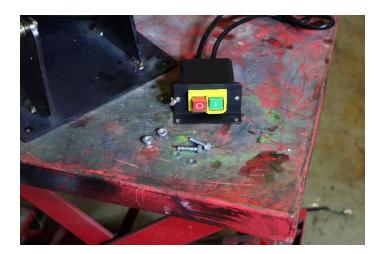
18. Mount switch using M6x20 bolts, washers and flange nuts.
