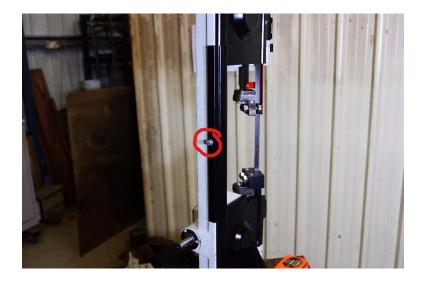
23. Loosen lower blade guide, move to upper most position, tighten.
