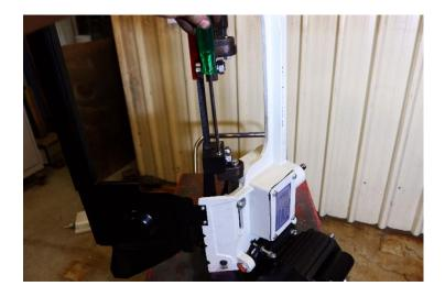
25. Loosen blade tension by turning the tension hand screw anticlockwise until the blade can be manipulated easily.
