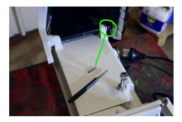
4. Loosen grub screw with allen key.
